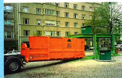
Filled Refuse Container being removed
